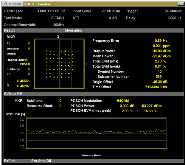
Figure 17 Measured EVM = 2.73%, CA 25km.
