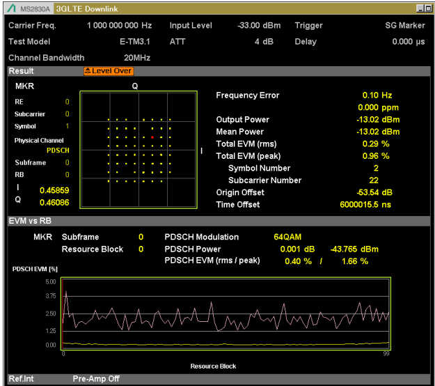
Figure 1 Base line EVM using 50cm or coax cable. RF power -12dBm.
