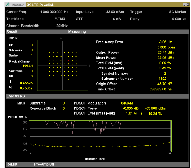
Figure 15 Measured EVM = 0.89%, CA 50cm coax.
