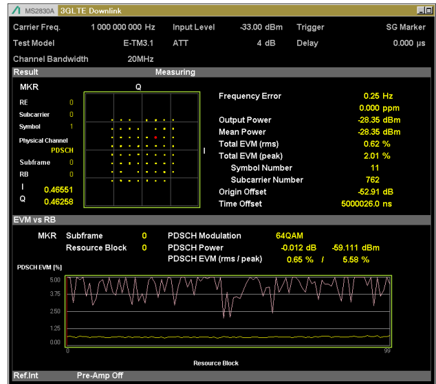
Figure 5 EVM for RFoF LTE base line measurement using 1m fiber. RF power -15dBm. Optical power 12.5 dBm.
