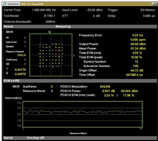
Figure 21 Measured EVM = 3.03%, CA 71km.
