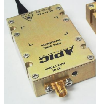
Figure 23 Picture of the used transmitter. Supply power 5V. Dimensions 40x64x15 mm 3 .
