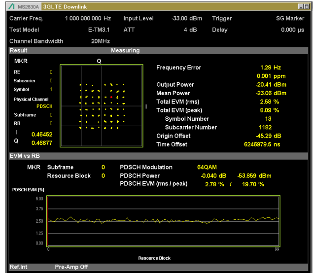
Figure 19 Measured EVM = 2.58%, CA 50km.
