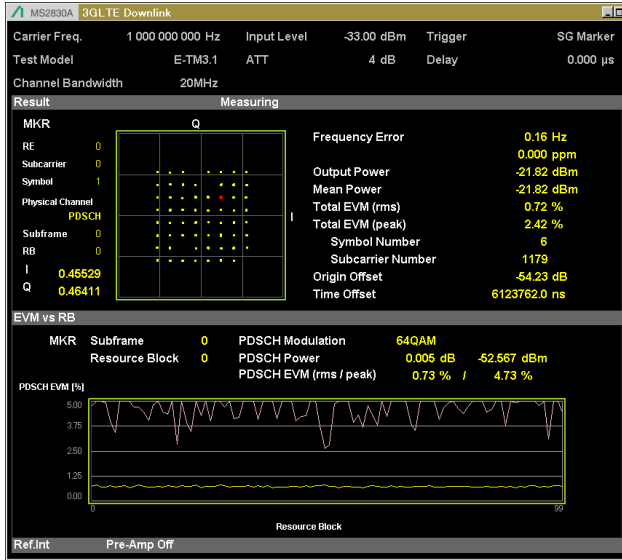
Figure 9 Measured EVM = 0.72% for 25km fiber.
