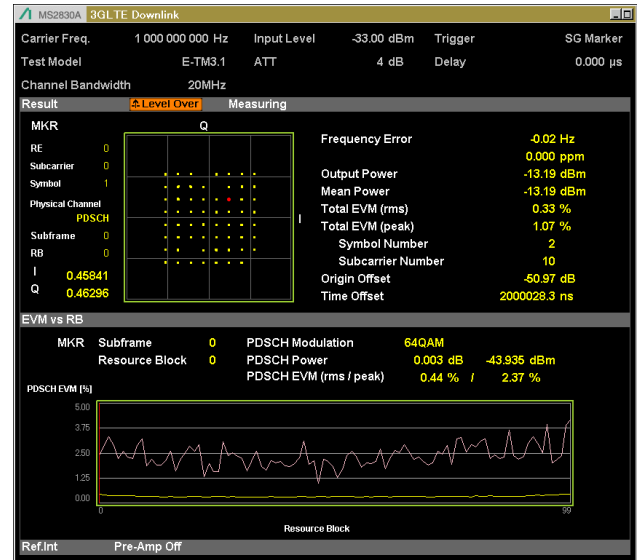
Figure 3 EVM for RToF LTE base line measurement using 1m fiber. RF power 1dBm. Optical power 12.5 dBm.
