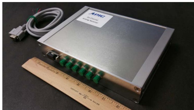
APIC Corporation's custom designed 6-Channel 20 GHz Analog Receiver
